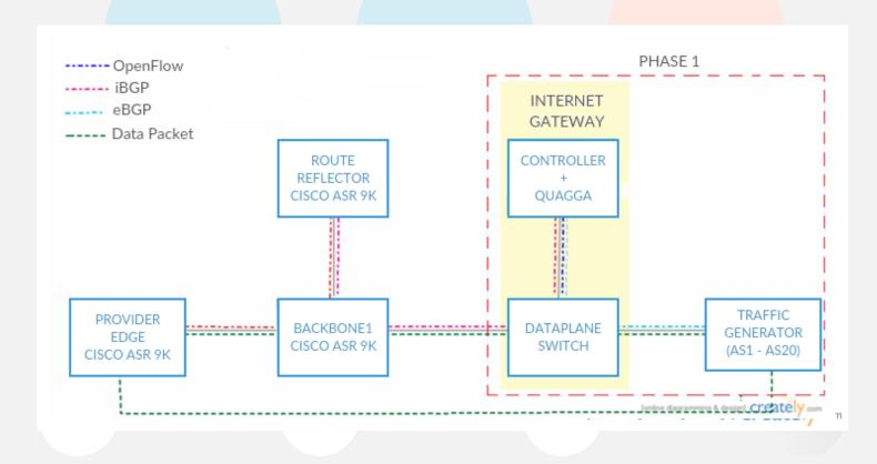
To ensure identical test conditions, all controller distributions are hosted on identically configured virtual machines. VMWare (ESXi 5.5.0) with a base Linux distribution of Ubuntu 14.04 is used in the test configuration. Quagga 0.99.24.1 and 0.99.22.1 with SDN controllers ONOS (1.5.0) and OpenMul (5.10.20) respectively, provide the control plane function. IXIA and Spirent emulate route updates from the internet peers.
