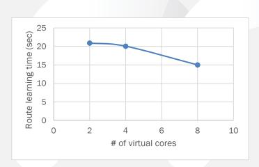
It was observed that that the performance is optimal when 6 or more virtual cores are allocated to the virtual machine that hosts Quagga. Given that in a Quagga + SDN Controller test scenario the same hardware resources will need to be shared by both the router and controller, it was decided to allocate <u>8 virtual cores for control plane VM</u> in the test-bed.
